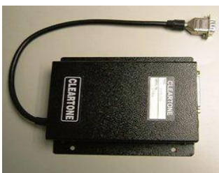
DM2 alarm / monitoring unit
